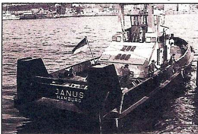
The HMS engine and thruster package can be easily lowered on to the barge deck and the drive legs tilted downwards to provide almost instant propulsion.
